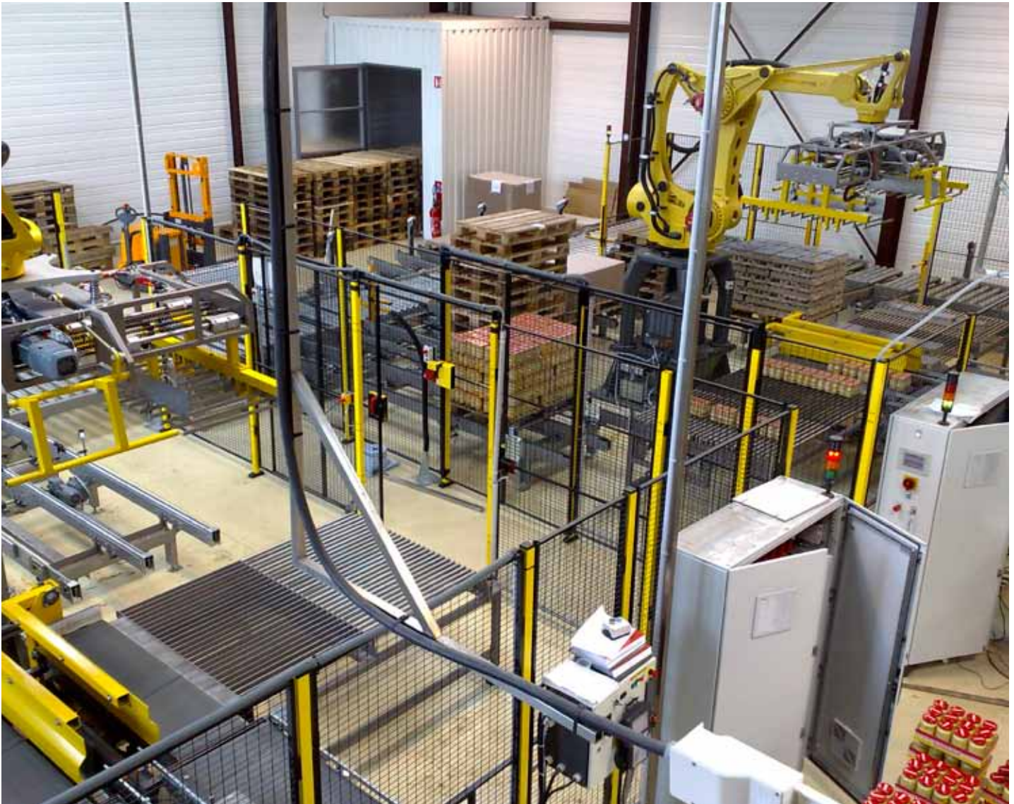
Axelent X-Guard®, height 2300 mm. The pictures show 25 metres of machine guard around a robot and pallets.
